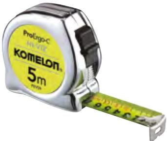
RUBAN ÉPAISSEUR 0,16 MM AVEC REVÊTEMENT HAUTE VISIBILITÉ (HI-VIZ). RUBAN AVEC PROTECTION NYLON. MESURE COMPACTE. BOÎTIER ABS CHROMÉ. AVEC BLOCAGE ET CLIP CEINTURE. ÉQUERRE 2 RIVETS POUR LE 3M, 3 RIVETS POUR LE 5M + RENFORT INOX.
