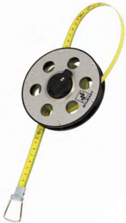
PROTECTION ABS SUR LA PÉRIPHÉRIE. BOÎTIER EN ALUMINIUM ANODISÉ. MANIVELLE ABS ESCAMOTABLE. RUBAN JAUNE ACIER LARGEUR 13 MM +FIBRE. LE 0 EST À LA BOUCLE CROCHET. LES OUVERTURES DANS LE BOÎTIER PERMET D'ÉVACUER FACILEMENT LES SALISSURES. GRADUATION EN MM UNIQUEMENT SUR LE BAS.
